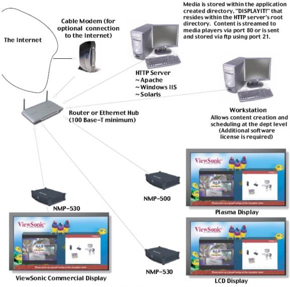
HTTP and ftp protocols are used to send and receive data to the Network Media Players. Commands are sent via port 80. Data is streamed back to media player from server via port 80. Static IP addresses for the server and Network Media Players are suggested to prevent "losing" displays after power interruptions. Revision 2.0 and later of DisplayIt! also uses port 21 to transmit data to and from the media player via ftp protocol.
